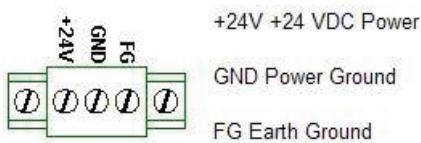
To make a connection, strip about 3/8" of insulation off the end of the wire, turn the connector screw counterclockwise until the gap is wide open, insert the wire all the way in, and turn the screw clockwise until it's tight.
