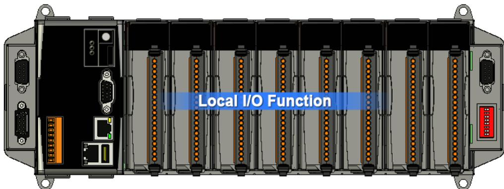
In the local mode, the slot range is from 0 to 7, the same the iSlot as follow.
