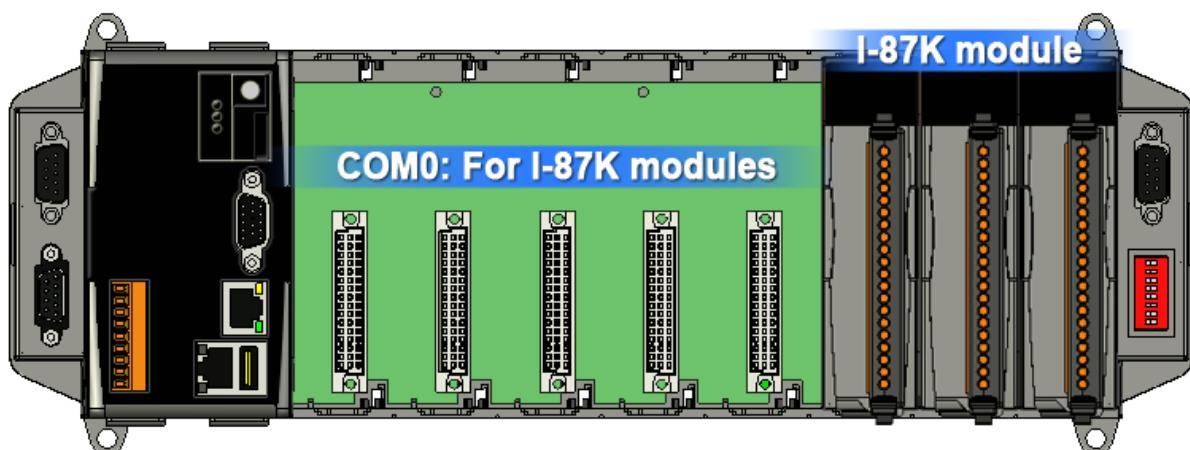
When a high profile I-87K is plugged in slot, please call the function, pac\_ChangeSlot, to change to the specific slot before doing other operations. Please refer to demo “87k\_Basic”.
