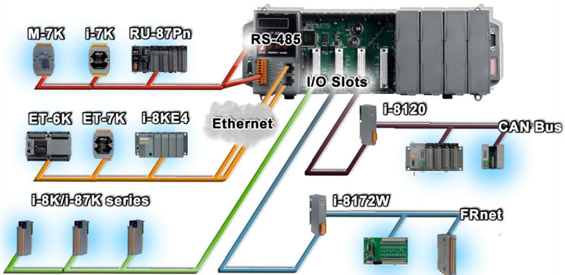
Beside the local I/O slots, iPAC-8000 also equips several RS-232/485 ports, two Ethernet ports to connect serial I/O and Ethernet I/O. And with FRnet and CAN communication module in local slot, FRnet I/O and CAN devices are easy to be integrated.
