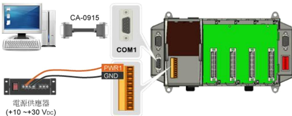
If the PC/Laptop is not fitted with a COM port, you can use the I-7560 (USB to RS-232)
