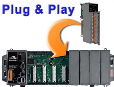
The iPAC-8000 features hot swap which means that there is no need to power off the iPAC-8000 for replacing modules. And the OS provides a function sending plug-in and removing messages to user's applications. Using this feature, users can design its own plug-and-play applications.
